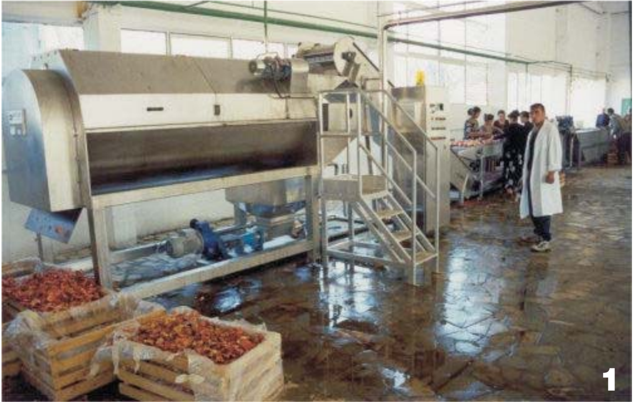
Picture 1: View of a complete squeezing group mod. ME-GRA included in a complete plant for pomegranate processing (capacity 5 tons / hour input) and supplied in Uzbekistan.
