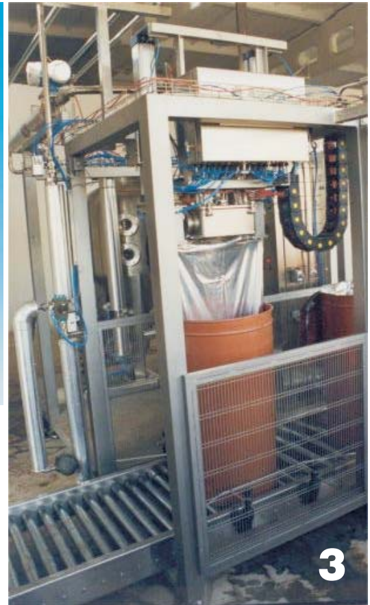
Picture 1 - Aseptic filler mod. C.A.F. 2H/1" -2" equipped for 220 l drums.
